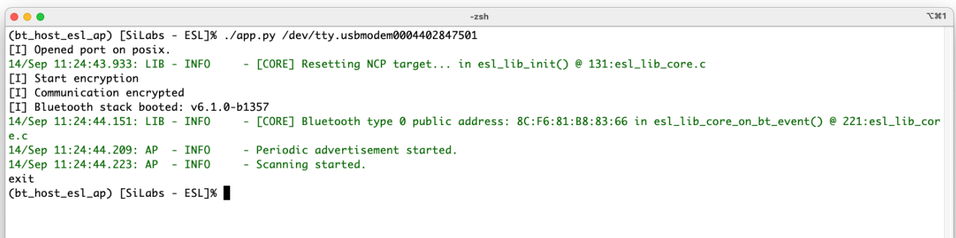
Figure 11. Start the access point with command python app.py <serial device> .
